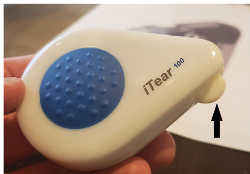
Figure 3. Commercial iTEAR100 device. The arrow denotes the oscillating tip with curvature and edge designed for chronic repetitive stimulation of the external nasal nerve.
